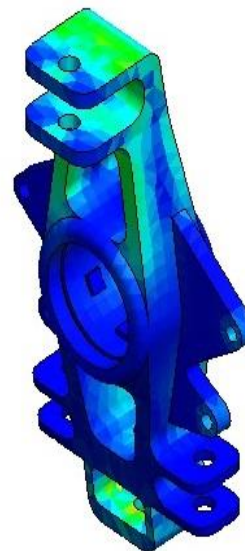
Fig. 6 Front Upright Strain Plot
