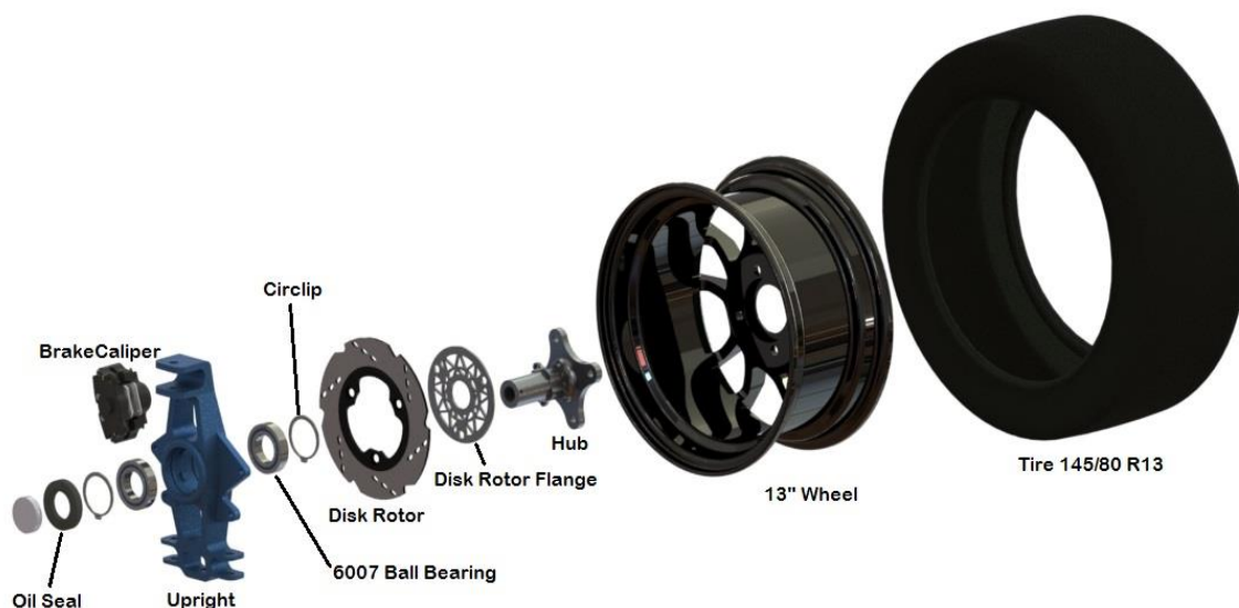
Fig. 12 Final Upright Assembly
